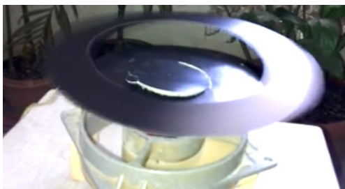
Pic.7. Rotation of the annular flat ring by the centrifugal up-stream.
